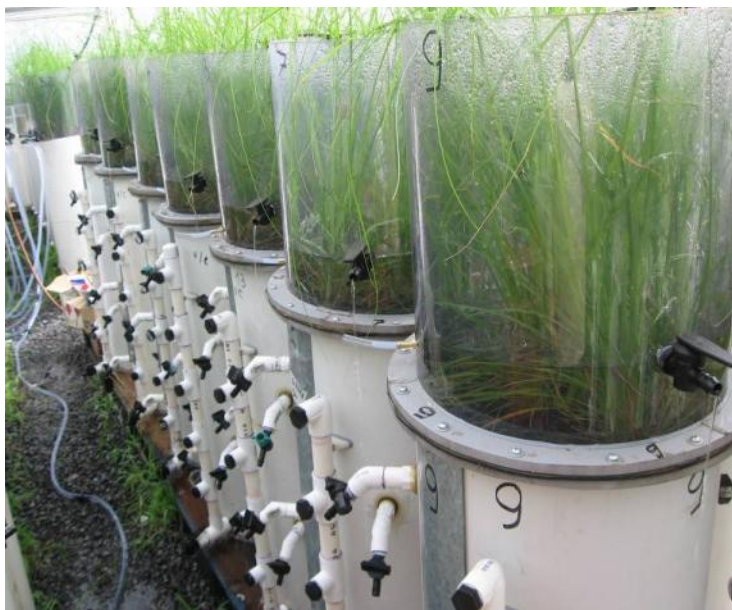
Testing the impact of a submerged zone, carbon source, and variable wetting and drying in the advanced columns
