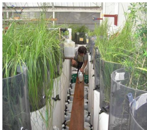
Laboratory biofilter column experiments: (LHS) non-vegetated soil filter media columns and (RHS) standard columns
