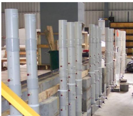
Laboratory biofilter column experiments: (LHS) non-vegetated soil filter media columns and (RHS) standard columns
