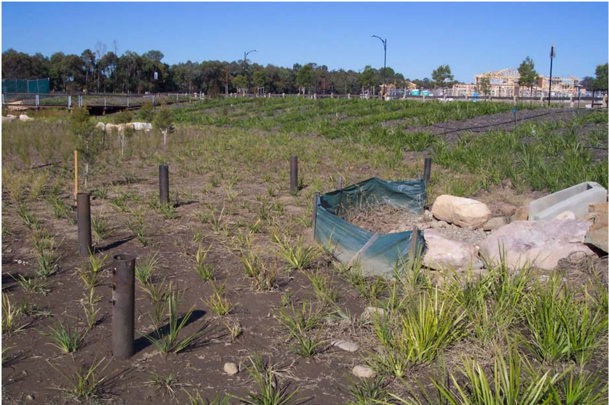
Figure S3.4 Metal columns installed at Second Ponds Creek bioretention installation and used in testing the hydraulic conductivity of the filter media.
