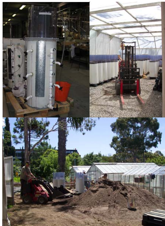
Preparation of bioretention experimental columns
